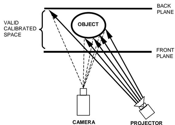
Fig 1. Experimental setting. The camera and projector situation are presented; and also the back and front planes.
