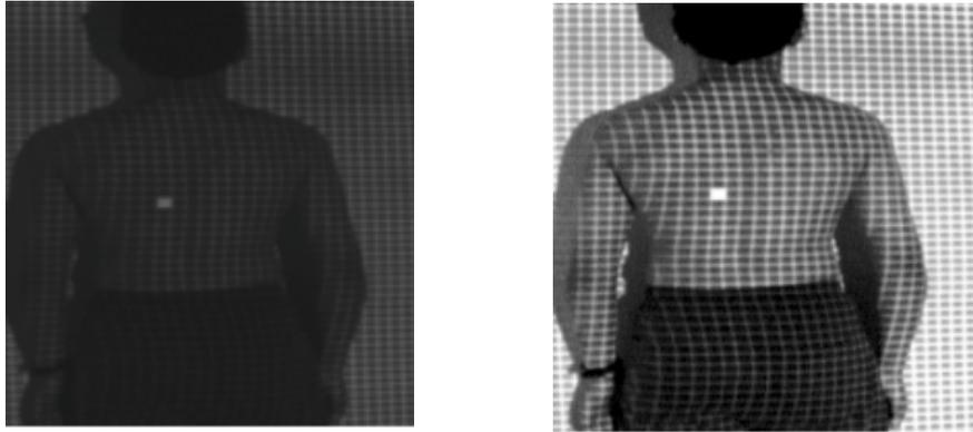
Fig. 5.a (left) Image of the back with the projected net as it is digitized; 5.b (right) The same image but equalized in order to make the pattern lines evident.
