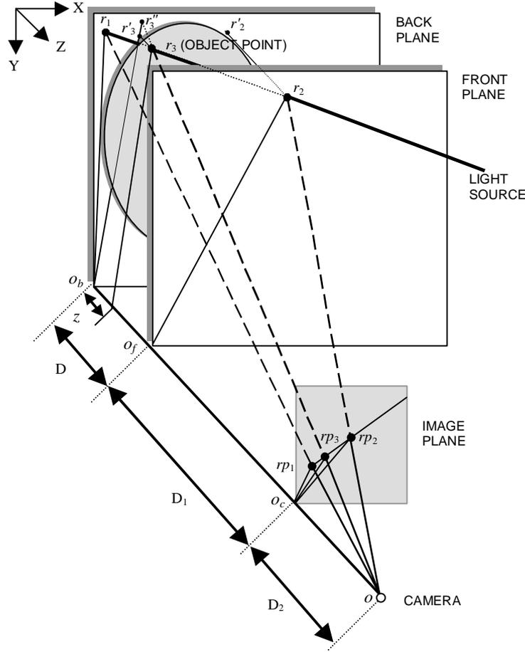
Fig. 2. Representation of the intersection points between a light beam and the front plane, the object surface, and the back plane. In addition, the positions where those three points are imaged are also displayed.
