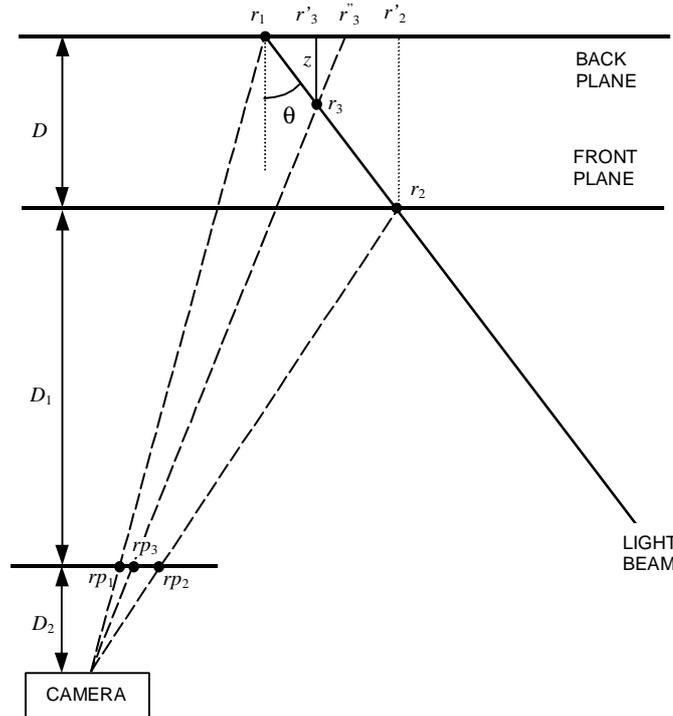
Fig. 3. (an upper view of Fig.2) Relations between the projection angle,  $\theta$ , and the distances to the image plane.
