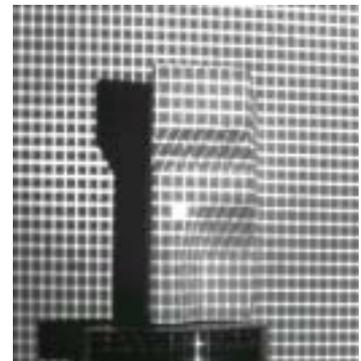
Fig. 4. Projection of the net on an object with steep slopes and with uneven textures in those zones.
